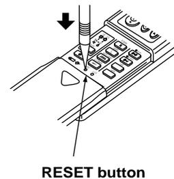
**NOTE :** If the RESET button is not pressed, the remote controller may not operate correctly.
